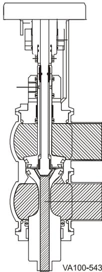
**Figure 17 - Lower Seat Lift for W71**
