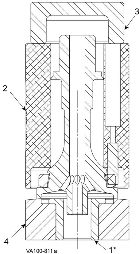
**Figure 33 - Lower Stem Tef Flow<sup>®</sup> P Seat Removal (Kit # 132947+)**
