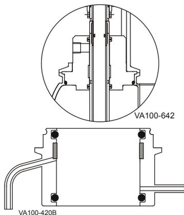
Figure 8 - External Steam Barrier - upper stem
