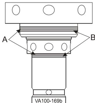
**Figure 18 - Adjustment zones with scribe lines**
