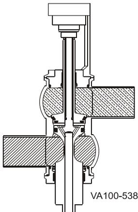
**Figure 14 - Valve Closed**
