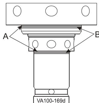
**Figure 19 - Bottom edges align with scribe lines**
