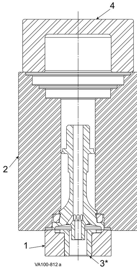
**Figure 34 - Lower Stem Tef Flow<sup>®</sup> P Seat Installation (Kit # 132357+)**
