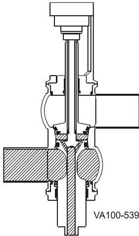
**Figure 16 - Lower Seat Push for W72RS Series**
