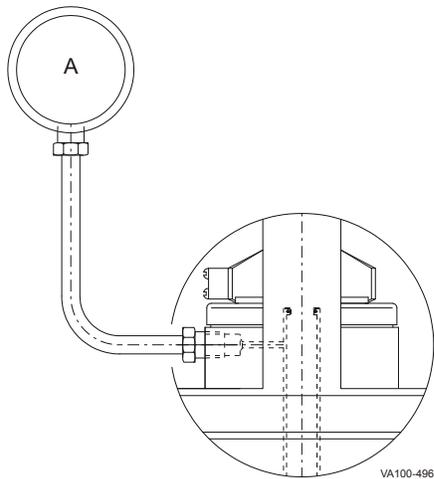
Figure 7 - Connection of Flush Supply
