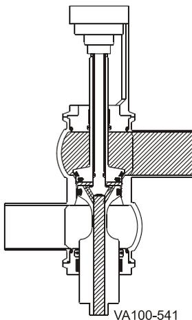
**Figure 15 - Valve Closed, Upper Seat Lifted**
